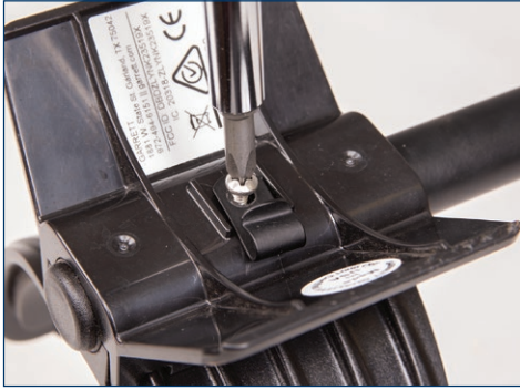
1. Remove screw and metal clip beneath detector stand.
