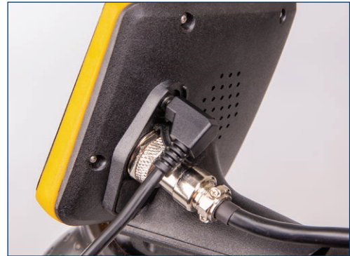
5. Plug adapter into 1/8" headphone jack on back of control box.
